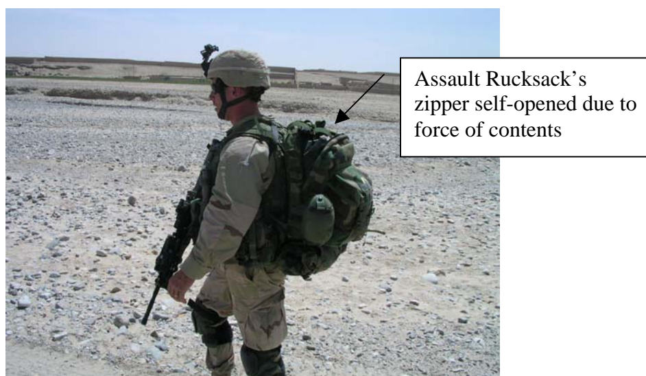
Figure B.2 Soldier's Assault Rucksack Zipper Has Self-Opened
